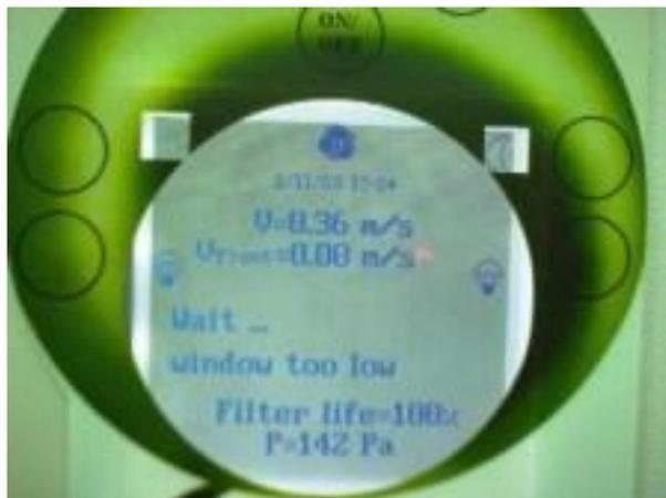
When the cabinet comes back to the normal use, the sash window stays closed until the velocity is OK. Then, the window raises itself to the correct height.
