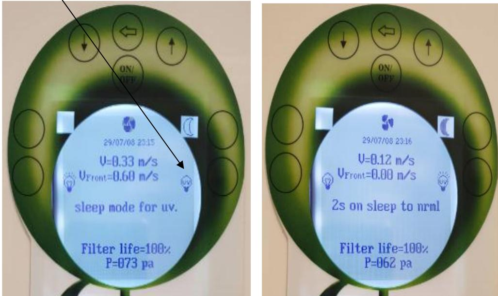
When the UV lamp is on, small rays appear on the screen logo. The UV lamp switches off automatically after the programmed duration (factory setting: 30 minutes). Can be modified in the "UV duration" section of the user menu.
