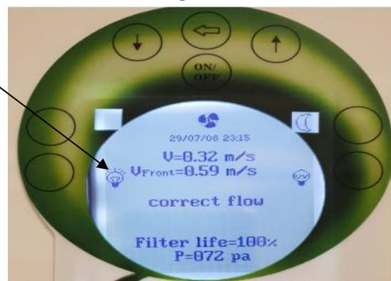
**UV (according to the models):** Press the UV button to turn the UV lamp on or off. The UV lamp can only be turned on in standby mode. If the device is in normal mode, the message “Standby mode for UV” appears
