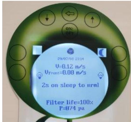
To switch from standby mode to working mode, press the button
