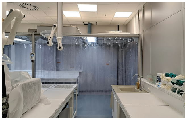
IPS Classe ISO 6 Gigafactory batteries
