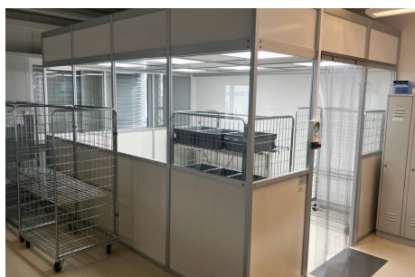
HPL walls with polycarbonate and vinyl curtains
